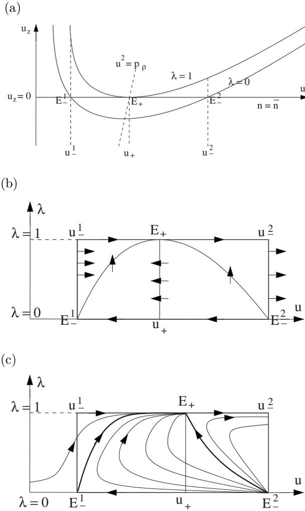
FIG. 8. (a) shows  $u_z$  as a function of  $(u, \lambda)$  for a fixed  $n = \bar{n}$ . The arrows in (b) illustrate the signs of  $u_z$  in the  $(u, \lambda)$  coordinates. A one-dimensional family of layer solutions connecting  $E_-^2$  to  $E_+$  is plotted in (c). Those solutions are bounded by layer solutions  $E_-^1 \rightarrow E_+$ ,  $E_-^2 \rightarrow E_+$  and the wet shock  $E_-^2 \rightarrow E_-^1$ .
