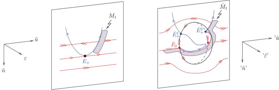
FIG. 12. A sketch of the supersonic slow manifold  $M_1$  of the extended system  $\{(5.3), \epsilon_z = 0\}$  in  $(\tilde{u}, \tilde{n}, \epsilon)$ -space (left). The blow-up of the region near the fold surface (black-dot, left) and a sketch of the extension of the slow (blown-up) manifold  $\hat{M}_1$  over the blown-up sphere (right).
