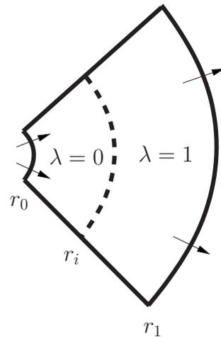
FIG. 2. Spherically symmetric nozzle geometry: the cone's boundary is shown in solid bold. Fluid is injected at  $r = r_0$  and discharged at  $r = r_1$ . The dashed curve at  $r = r_i$  indicates an internal boundary layer of a standing evaporation wave where a transition from a liquid state ( $\lambda = 0$ ) to a vapor state ( $\lambda = 1$ ) happens.
