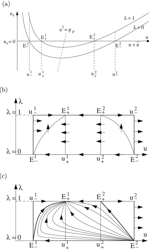
FIG. 7. (a) shows  $u_z$  as a function of  $(u, \lambda)$  for a fixed  $n$ . The arrows in (b) illustrate the signs of  $u_z$  in the  $(u, \lambda)$  coordinates. A one-parameter family of layer solutions connecting  $E_-^2$  to  $E_+^1$  is plotted in (c). Those solutions are bounded by layer solutions  $E_-^1 \rightarrow E_+^1, E_-^2 \rightarrow E_+^2$ , the wet shock  $E_-^2 \rightarrow E_-^1$ , and the dry shock  $E_+^2 \rightarrow E_+^1$ .
