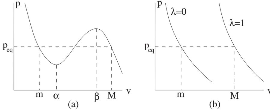
FIG. 1. (a) shows the van der Waals pressure function  $p(v)$  where the Maxwell line  $p = p_{eq}$  connects  $v = m$  to  $v = M$  on  $p = p(v)$ . (b) shows the functions  $p(\lambda, v)$ ,  $\lambda = 0, 1$ , where the Maxwell line  $p = p_{eq}$  connects  $v = m$  on  $\lambda = 0$  to  $v = M$  on  $\lambda = 1$ .
